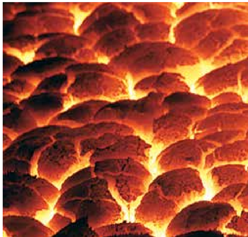
Coke is a fuel that rose to prominence in western Pennsylvania during the 1800s, and is derived from coal, having its impurities removed in order to increase its carbon content.
